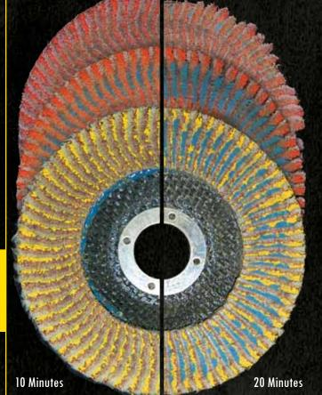
Flap discs provide the added benefit of finer finishing after aggressive grinding, compared to resin fibre discs. The dimensional layering of flap discs allow the continual exposure of abrasive grains, versus one layer of grains. Flap discs contain just as much working surface as resin fibre discs, but within a much smaller diameter. This geometry is responsible for the versatility of a flap disc. The integrated grinding aids utilized in
