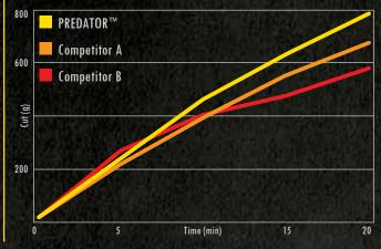
After a 20 minute automated grinding test, our PREDATOR™ flap disc cut over 100 grams more than the next leading competitor. Although the disc may look worn, it continues to cut for extended periods of time.
