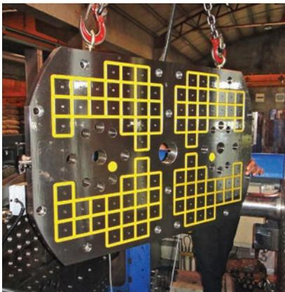
Load and install PIM magnet with bolts
