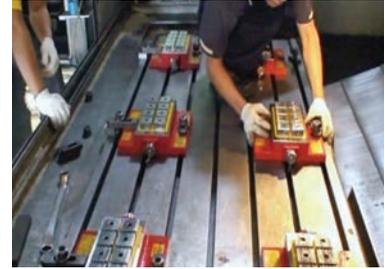
Position the chucks on the machine bed.
