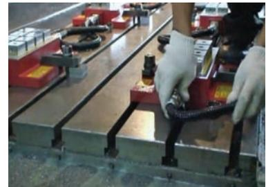
Connect the control cables to chucks and control
