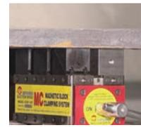
Use EEPM-SP spring-loaded induction blocks and EEPM-SPF blocks together to hold warped stock. See page 243.
