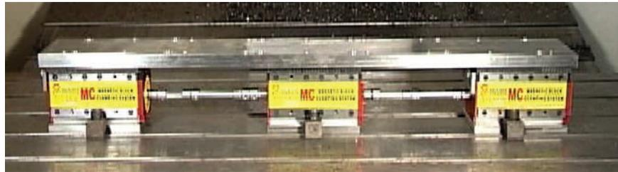
Switch-connect ECB vises to turn ON/OFF simultaneously
