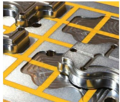
For machining small, thin, or irregular parts that do not have much metal to attract the magnet, you can create a shallow nest, or pocket in a subplate or induction blocks to secure the part and prevent lateral movement. For part nests that you will use over-and-over again on repeat jobs use subplates to save setup time.
