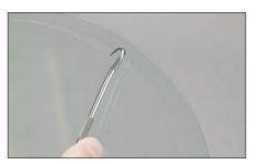
3.) Gently push the point of the Film Removal Tool between the top and next layer of the Scotchgard<sup>TM</sup> Protective Film and twist the tool to separate the two sheets. If working with single layer film without a stepped edge, near a corner, press the tip of removal tool against the film, pierce the film and twist the tool as to lift the film.
