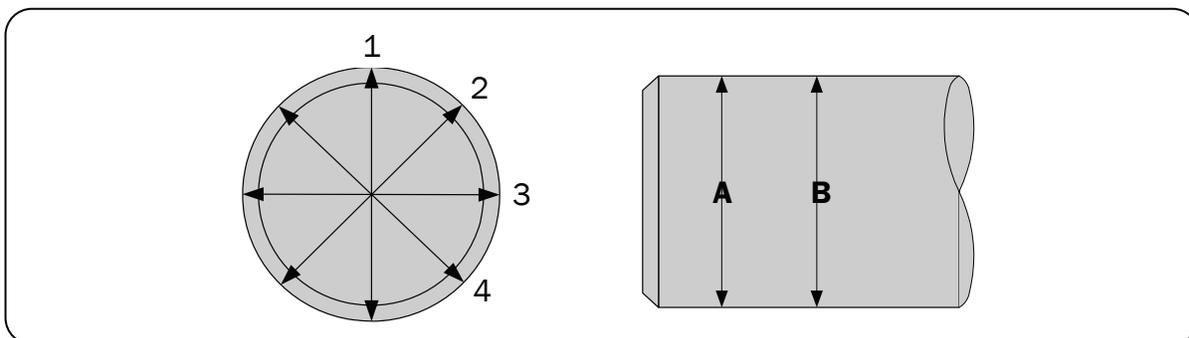
**Shaft Tolerances When Used with Adapter or Withdrawal Sleeves**
