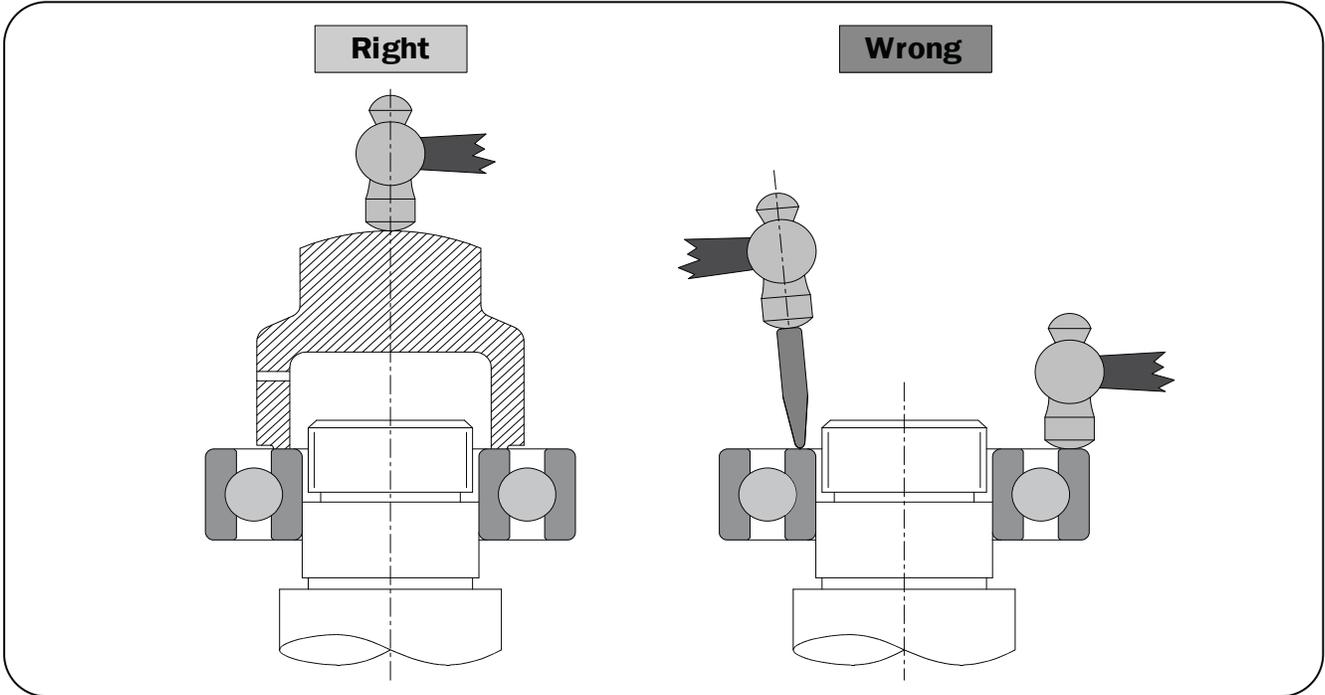
When you are mounting the inner and outer rings at same time, use a metal buffer and apply a force simultaneously on both rings.
