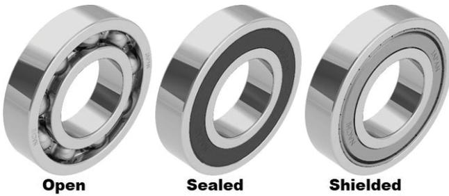
The capacity of a bearing will be the same regardless if is open, has seals, or shields. All three bearings will accept the same load and produce the same life. The three bearings will have different speed limits. Speed limits are determined by how hot the bearing will operate. The higher the
