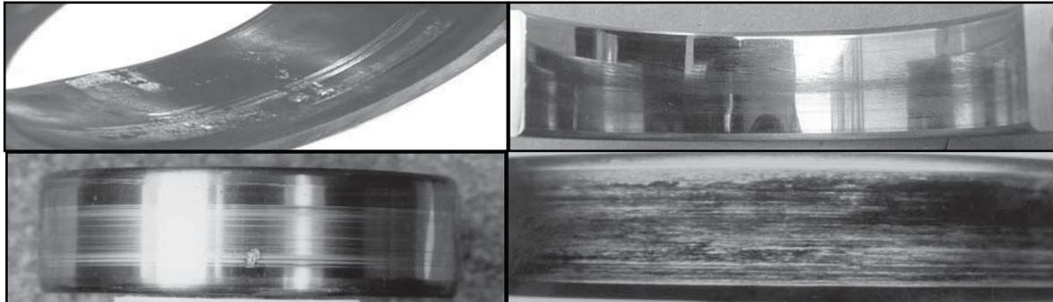
**Electric Arcing:** Pitted or corrugated surface caused by electric current pass.
