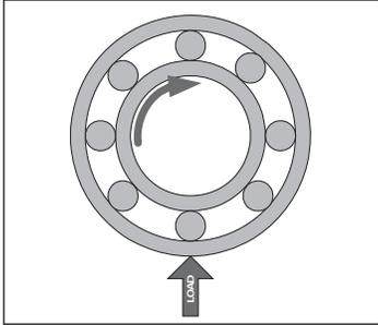
The shaft rotates and the direction of the load does not change. The outer ring is stationary. The entire inner ring raceway comes under load during one revolution of the shaft. Only a portion (an arc) of the outer ring comes under load. This is the most common application. Example: Electric Motor
