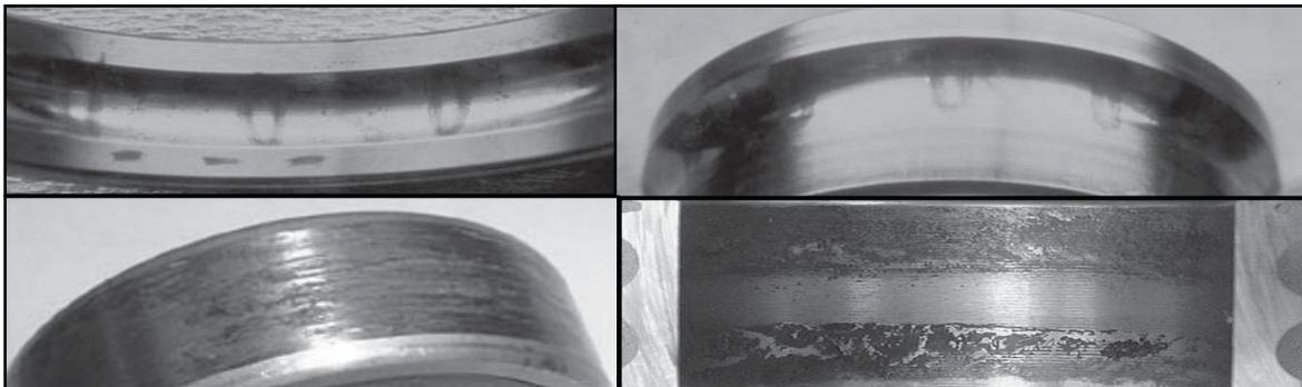
**Smearing:** Metal to metal contact due to the destruction of oil film. Sliding between outer ring, inner ring and rolling element.
