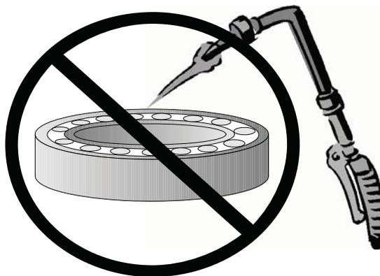
When using an oil bath heating tank, place the bearing on a screen that is several inches off the bottom and heat the tank to the required temperature. Normally good quality machine oil or transmission oil is used.
