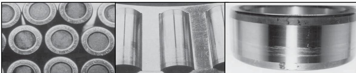
**Excessive Wear:** Surface deterioration due to heavy sliding friction between the contact areas of the bearing components
