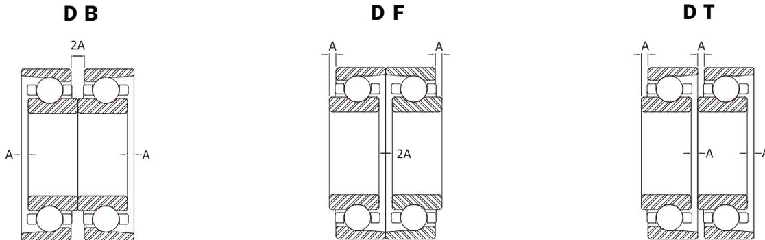
These sets of two bearings have been selected as matched pairs at the factory. One DU set of bearings has only a small dimensional variation ( $2\mu\text{m}$  maximum) on the bore diameter and OD of the two bearings. The dimensions are shown on the inspection sheet in the box and on the side of the box. Each bearing is serialized.
