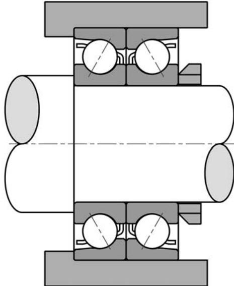
On “DF” arrangements the outer ring must be clamped to preload the bearings.
