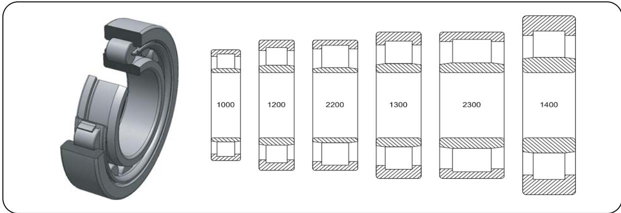
For each size there are many ring configurations (types) as shown below. The type depends on the ribs on the inner and outer ring. The most common types are the NU and NJ. NU has two ribs on the outer ring and no ribs on the inner ring, this type cannot accept thrust load. This configuration is often used as an expansion bearing. The NJ has two ribs on the outer ring and one rib on the inner ring, this type can accept a small thrust load in one direction.
