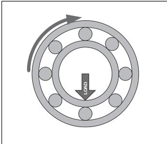
The shaft remains stationary and the outer ring rotates. The direction of the load does not change. The entire outer ring raceway comes under load during one rotation of the housing. Only a portion of the inner ring raceway ever comes under load. Example: Pulley
