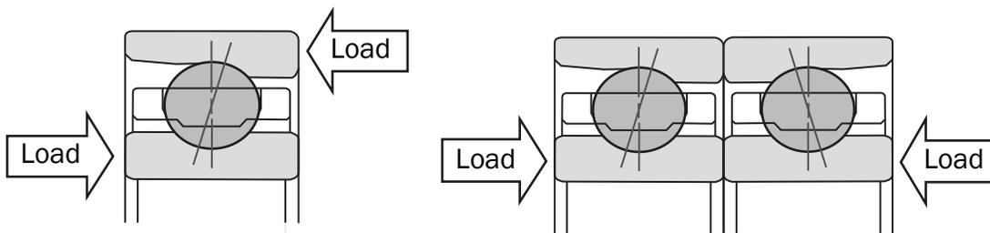
**Single row angular contact bearings can only be loaded in one direction.**
