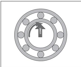
The shaft rotates and the load rotates with the shaft. The outer ring does not rotate. The entire outer ring raceway comes under load during one rotation of the shaft. Only a portion of the inner ring ever comes under load. Example: Vibrating Screen
