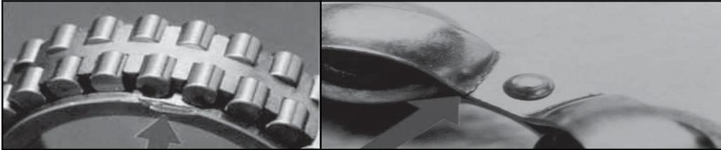
**True Brinelling:** The occurrence of dents on the raceways that are the result of exceeding the elastic limit of the steel.
