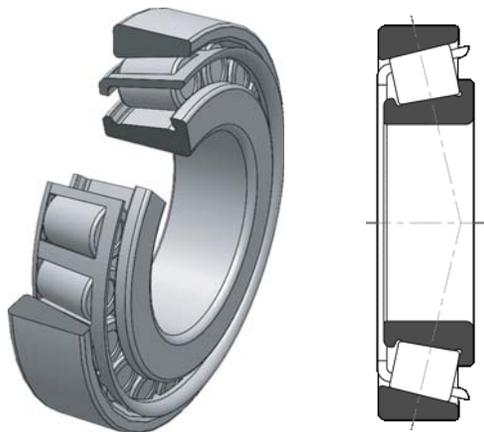
Thin section, high strength, stamped steel cages maximize the lubrication flow, which improves the lubrication factor resulting in longer bearing life.
