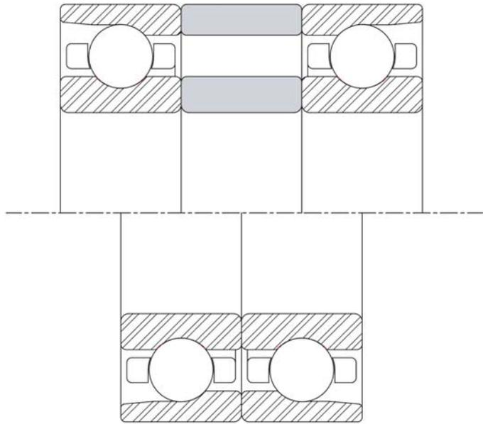
Angular contact ball bearings at the fixed end have tight fit and shoulder on the housing or shaft. Bearings at free end are cylindrical roller bearings or bearings which are not fixed in the axial direction. Therefore, they can move in the axial direction and they do not carry axial load. The float end is also the expansion end.
