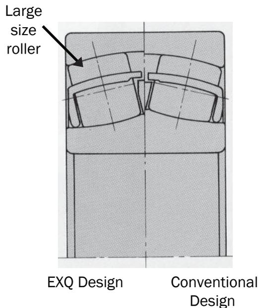
A special variation of spherical roller bearings for vibrating screen applications is detailed on Page 77 of this training guide.
