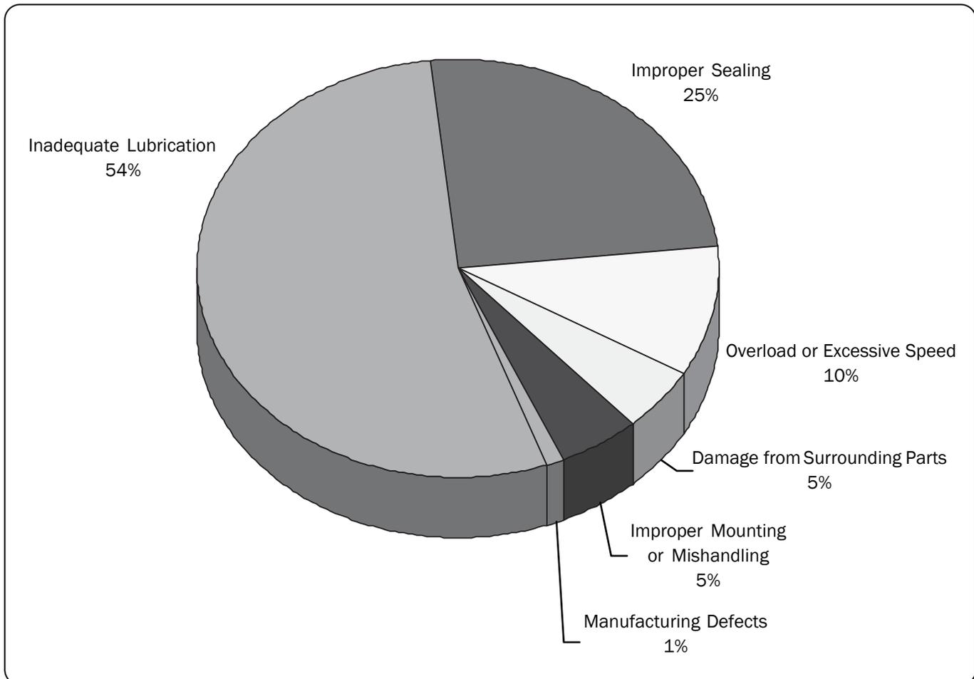
The majority of premature bearing failures are caused by inadequate lubrication. Anti-friction rolling element bearings are designed to have a thin film of oil between the rolling elements and the raceway surfaces. When this film degrades or gets too thin the rolling elements contact the raceway surfaces and wear develops. Anti-friction bearings are not designed to be wear parts.
