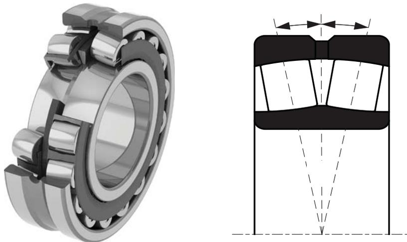
Double Row Spherical Roller Bearings are the work horse of the industry. Their spherical shaped outer ring and barrel shaped rollers permits this bearing to operate with 2° of misalignment with no reduction in bearing life.
