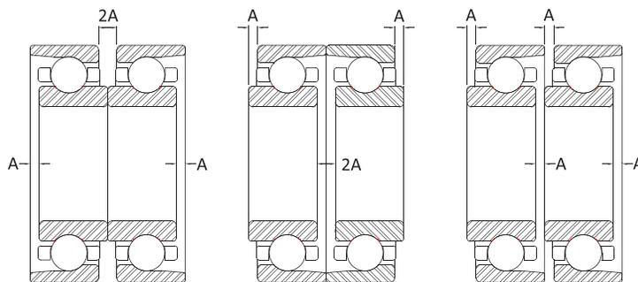
**Bearings** with the suffix “U” can be used in pairs. The inner ring and the outer ring have identical widths. This permits the bearings to be arranged in any combination such as back to back, face to face or tandem pairs.
