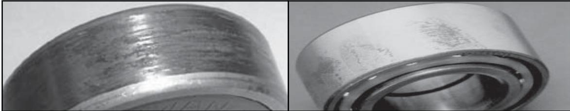
**Creep:** Galling, wear, sliding and discoloration of fit face.
