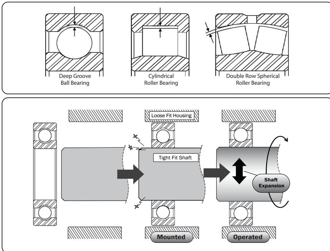
Country standards (ABMA, JIS, DIN) and international standards (ISO) for clearance ranges are the same. These clearance ranges will vary depending on type of bearing (Radial or Angular) and (Ball or Roller)
