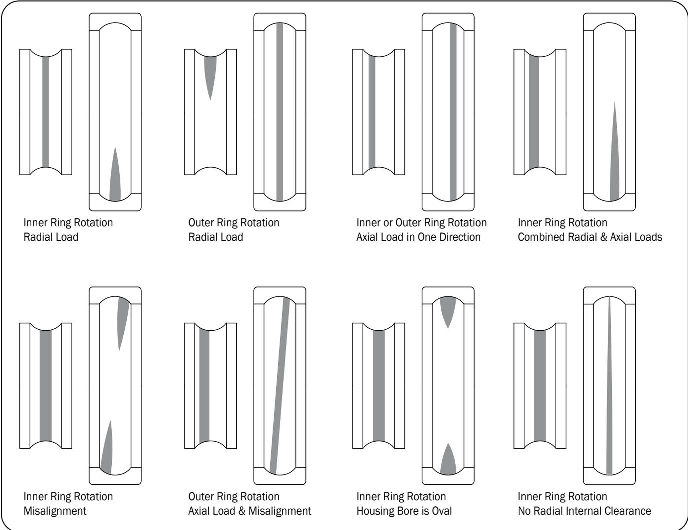
Bearings are like fuses, something causes the bearing to fail. We use these visual wear patterns to determine if the application is normal or if something is abnormal. By shining a bright light (Mag flashlight) down the raceway, these patterns pop out and become more visible.
