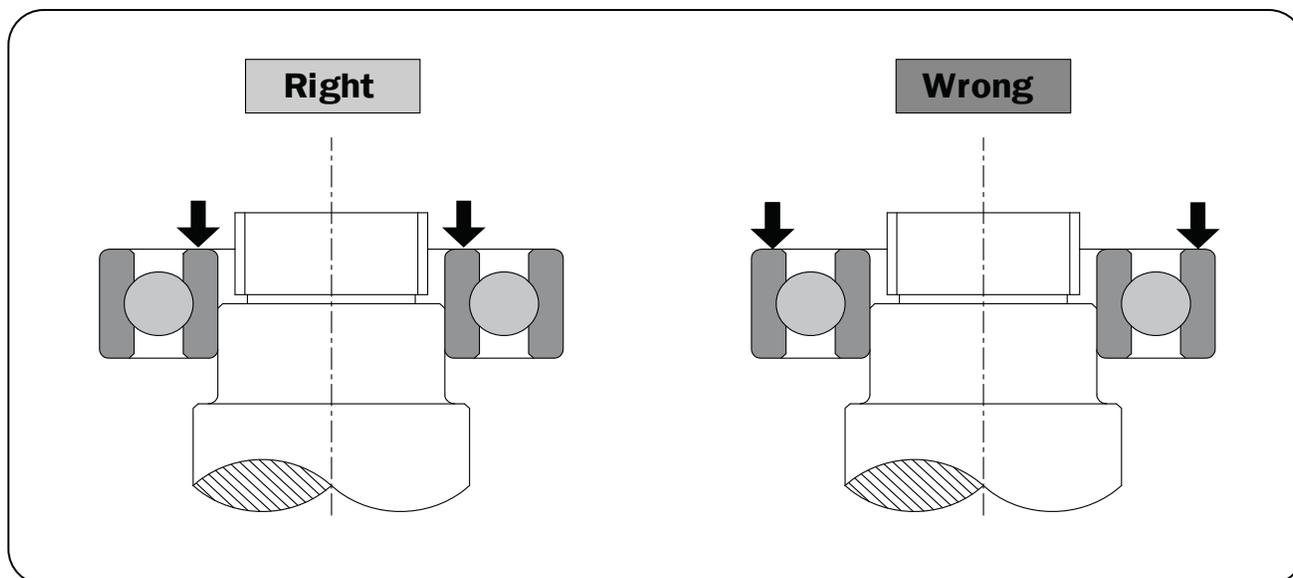
When force is to be applied on the rolling bearing for mounting, it must be applied in a straight line and evenly. Make sure that bearing is centered correctly.
