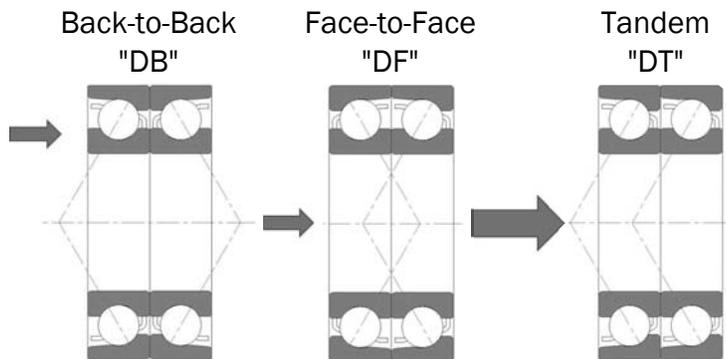
When bearing are used in duplex sets, or pairs, the bearings need to be special or matched sets. Bearings are very stiff and for both bearings to accept the loads evenly the bearings should be matched.
