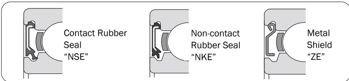
Nachi's design utilizes a groove in the inner ring and the seal contacts the side of the groove. Standard material for seals is Buna - Nitrile Rubber.
