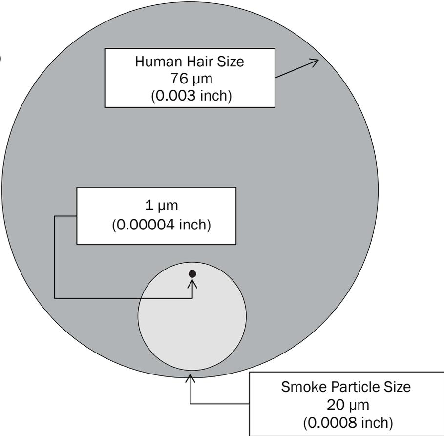
**Contamination in bearings is a constant problem.** Even a small amount of contamination will affect the bearings. A hair has a diameter of about 0.003" A smoke particle is 0.0008". Contamination the size of 1 micron is at least five times the film thickness of the oil on the raceways. The contour of the raceway surfaces are in the range of plus or minus 1 micron.
