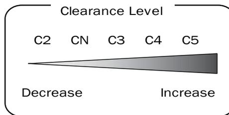
Application determines how much internal clearance should be in each bearing. This dictates how much clearance a bearing should have before installation. C2 Clearance is for slow application. CN is the standard clearance for the world. C3 is for high speeds and is standard in America. C4 is for high speeds and hot applications.
