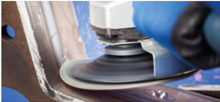
Particularly soft and flexible grinding properties for face-down grinding with fibre discs of diameter 125 mm.
