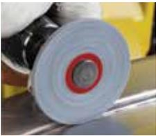
Finishing rough or pitted roof ditch brazes without slowing down the line can be a real challenge. Now you knock those brazes down to size, quickly and precisely – with new Scotch-Brite™ EXL PRO Unitized Wheels. These high
