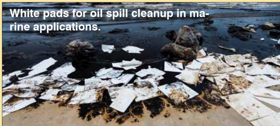
**White pads for oil spill cleanup in marine applications.**
