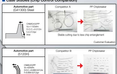
Stable cutting due to less chip entanglement
