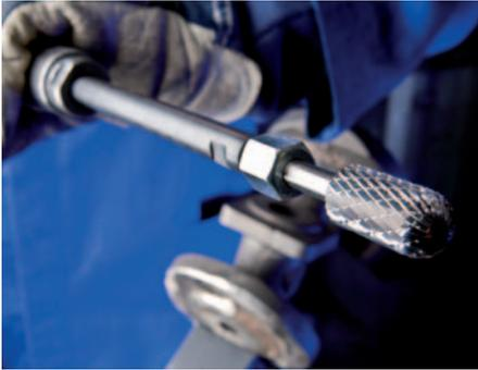
Burs (shank dia. 1/8" and 1/4") can be extended with spindle extensions, allowing access to hard-to-reach areas. The extension is mounted in the collet chuck of the machine (air-powered or electric), or in the handpiece of the flexible shaft. In some applications spindle extensions are efficient alternatives to customized burs with long shanks.
