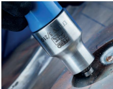
Conical counterbore burr for the production of precisely defined chamfers.
