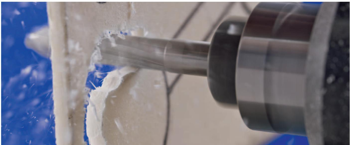
Bi-metal hole saws are used on drill presses and hand-held drills. Bi-metal construction ensures a long service life and high impact resistance for tough working conditions.
