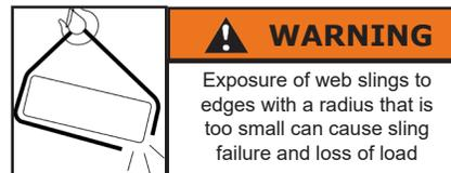
Edges do not need to be "sharp" to cause failure of the sling. Table 3-1 shows the minimum allowable edge radii suitable for contact with unprotected webbing slings. Chamfering or cutting off edges is not an acceptable substitute for fully rounding the edges to the minimum radius. Slings can also be damaged from contact with edges or burrs at the sling connections.
