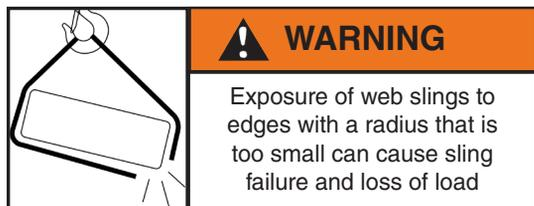
Edges do not need to be sharp to cause failure of the sling. The table shows the minimum allowable edge radii suitable for contact with unprotected webbing slings. Chamfering or cutting off edges is not an acceptable substitute for fully rounding the edges to the minimum radius. Slings can also be damaged from contact with the edges or burrs at the sling connections.
