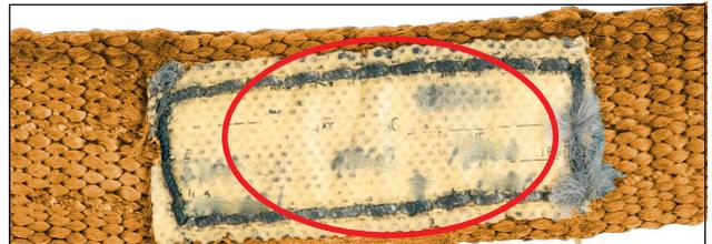
**Red Core Yarns** are an **additional** aid to warn of dangerous sling damage. All standard *Lift-All* Web Slings have this warning feature. The red core yarns become exposed when the sling surface is cut or worn through the woven face yarns. When red yarns are visible, the sling should be removed from service immediately. For other inspection criteria see OSHA/Manufacturer regulations in the HELP section of this catalog and the safety bulletin provided with each sling.
